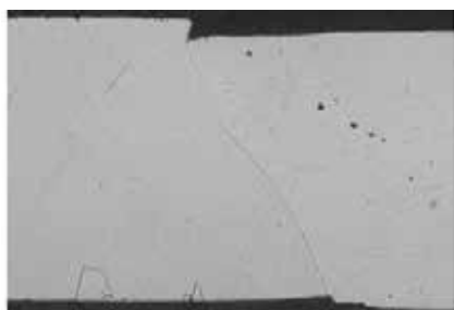
Micrograph of standard Pt wire after 6 hours at 1400 °C under a tensile stress of 2.76 Mpa, showing a large grain structure and resulting grain boundary movement.
